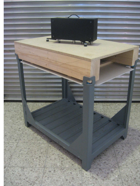
Figure 11: Construction of COMET, timber floor
