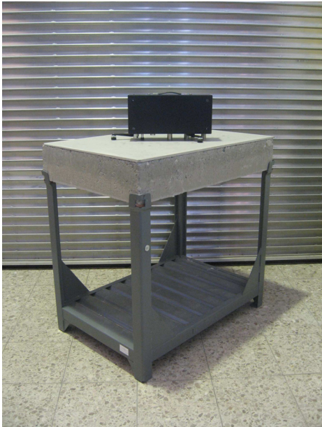
Figure 10: Construction of COMET, concrete floor
