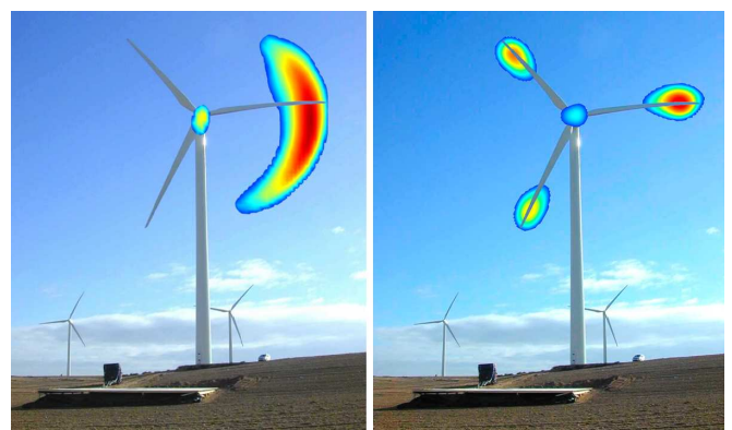
Figure 7: Wind turbine field test, post processing with stationary focus (left) and rotating focus (right).
