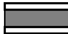
Figure 2: Cross section of the beam specimen: outer layers of aluminium, inner layer of silicone, symmetry in vertical direction
