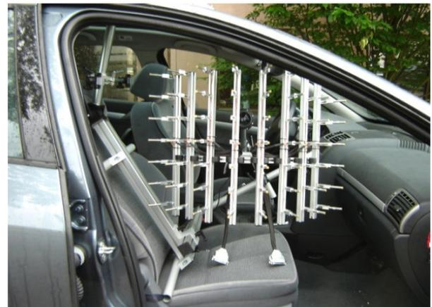
Figure 9: Half cylindrical array
