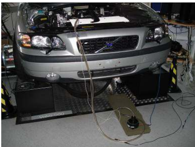
Figure 4: Mid-high frequency volume velocity source based on horn driver and flexible hose for measuring in-vehicle transfer function.
