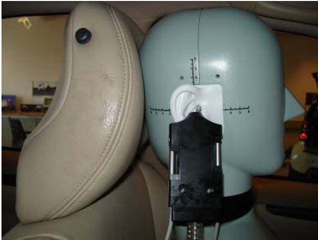
Figure 9: Positioning the adaptor of mid-high frequency sound source at HATS right ear for reciprocal transfer function measurements.
