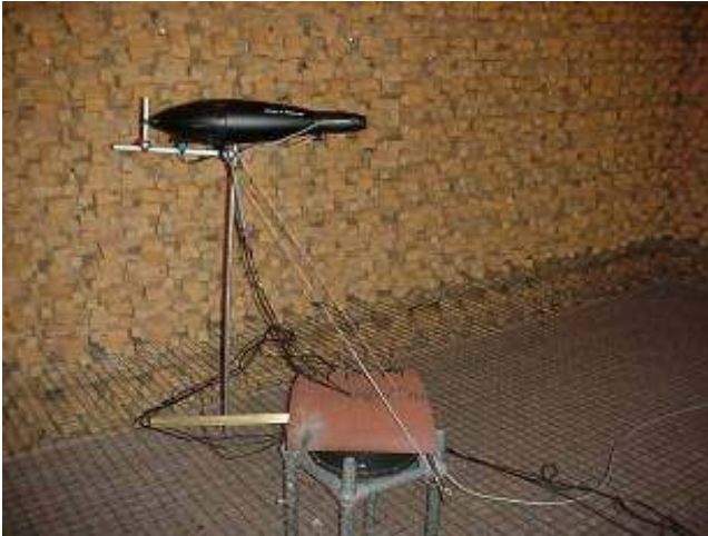
Figure 3: Low-mid frequency volume velocity source without hose in anechoic chamber.
