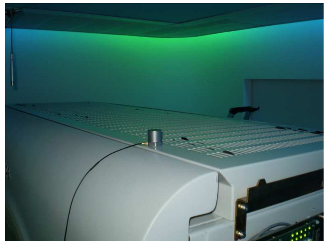
Figure 13: Accelerometer measurement set-up to determine the vibration levels of the CT gantry
