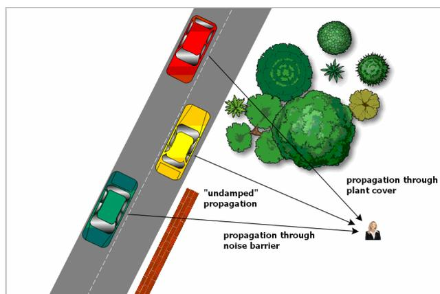
**Figure 2:** Depending on the investigated area specific damping filters must be calculated and applied to the source signals.
