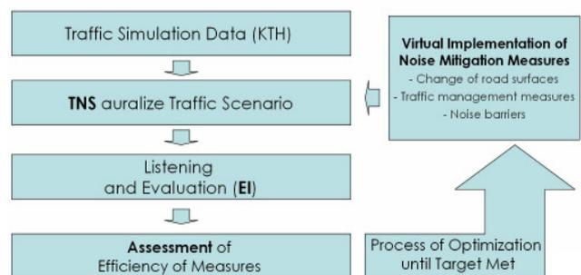
**Figure 5:** Schematic use of TNS for the assessment of virtually implemented mitigation measures
