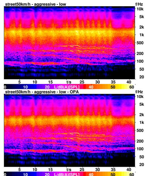
**Figure 4:** Auralized traffic scenarios: Noise of single street with low traffic volume and standard road surface (top) compared to same setting and same traffic volume with a low noise pavement (OPA) (bottom)
