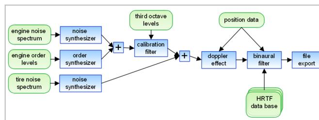
**Figure 1:** Part of the signal processing network: The green boxes represent the data coming from the source model or the traffic noise application. The blue boxes display calculation nodes and the arrows show the data flow.
