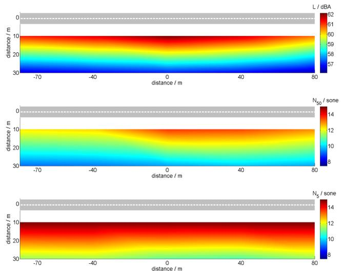
Figure 6: Noise maps of a single street with a traffic volume of 1400 vehicles/h displaying dB(A) (top), N<sub>50</sub> (middle) and N<sub>5</sub> (DIN) (bottom) [9]; distance in [m]
