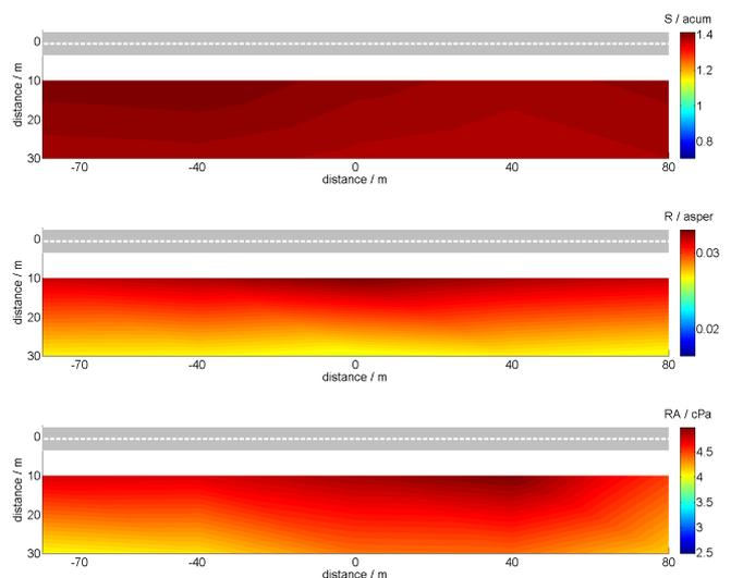
Figure 7: Noise maps of a single street with a traffic volume of 1400 vehicles/h displaying Sharpness (DIN) (top), Roughness (Hearing Model) [10] (middle) and Relative Approach (bottom) [11]; distance in [m]
