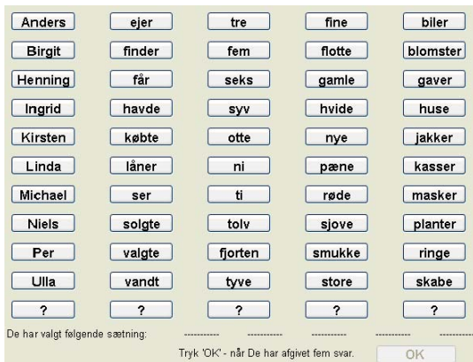
Figure 7: MATLAB user-interface employed in the speech intelligibility experiments and presented via a hand-held touch-screen. Listeners had to indicate the perceived words by pressing the corresponding buttons.
