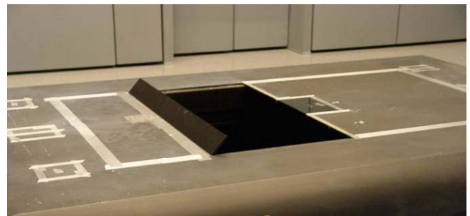
Figure 2: SAE Type 4 body: modular design of the sunroof opening and removable deflector [1]
