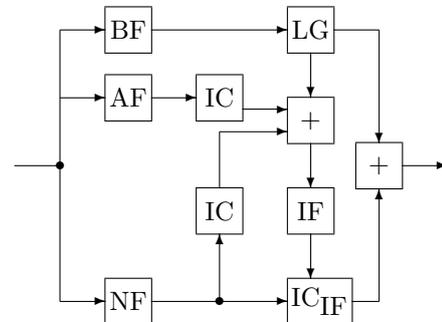
**Figure 1:** Block diagram of one frequency channel of the model. BF: Broadband filter, NF: Narrowband filter, AF: Additional narrowband filter, LG: Linear gain, IC: Instantaneous compression, IF: Instantaneous frequency estimation
