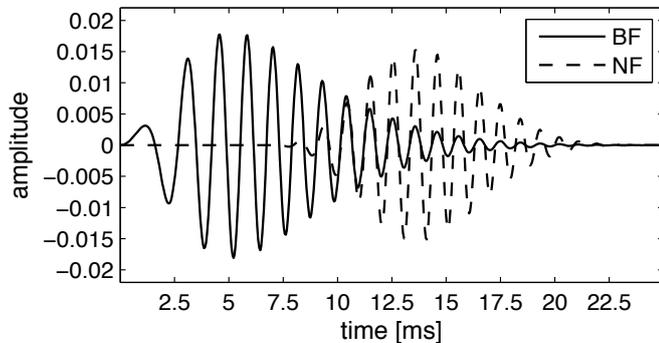
**Figure 3:** Impulse responses of the filters BF and NF.
