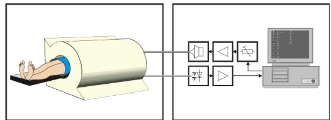
**Figure 1:** left: MRI operational room: 1.5 T scanner, standard head coil; right: Control room: PC, attenuator, amplifier, dynamic loudspeaker system, feeding into silicone tube (inner diameter 6 mm, length 12 m, top middle). Fibre-optical line (bottom middle) connects optical microphone (left, not shown) to control box (right) with light-to-voltage transducer.
