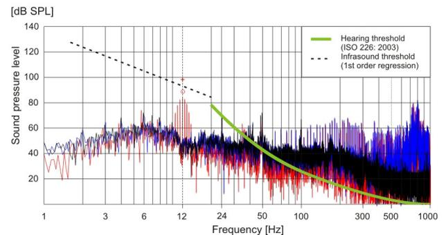
**Figure 7:** 12 Hz, 90 dB SPL test signal spectrum (red) together with noise spectra and thresholds as in Fig. 4. The red small circle at 12 Hz denotes the SPL value of the modulation line cluster around 12 Hz, the red asterisk denotes its peak equivalent SPL.
