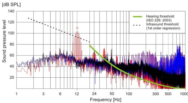
**Figure 8:** 12 Hz, 110 dB SPL test signal spectrum (red) together with noise spectra and thresholds as in Figure 4. The red small circle at 12 Hz denotes the SPL of the modulation line cluster around 12 Hz, the red asterisk denotes its peak equivalent SPL. Modulation line clusters around 36 Hz, 60 Hz, and 84 Hz represent harmonic distortion above normal threshold.
