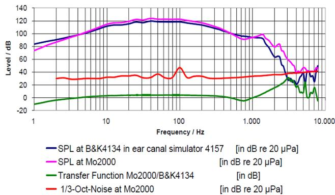
**Figure 4:** Steady-state frequency responses of microphones in-situ, as shown in Figures 2 and 3, with  $U_{RMS} = 1$  V at the loudspeaker
