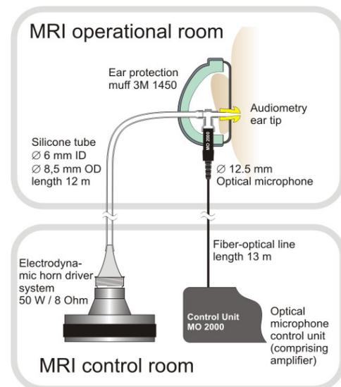
**Figure 2:** Sound coupling to the ear. Electrodynamic loudspeaker system (bottom left) feeding into silicone tube, through ear muff; into subject's ear (top right). Optical microphone (top right) is coupled via T-fitting to ear tip, its fibre-optic line is connected to control box (bottom right).
