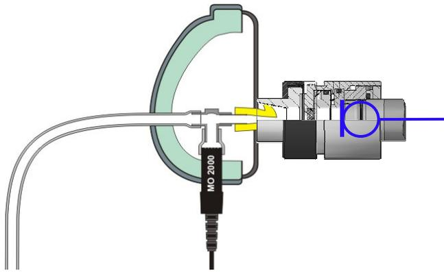
**Figure 3:** Calibration of optical microphone at the interface of sound tube and ear canal, using occluded-ear simulator B&K 4157 with built-in microphone B&K 4134
