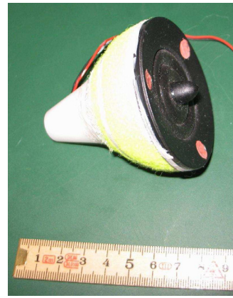
Figure 2: Source for free-field calibration used at DPLA.
