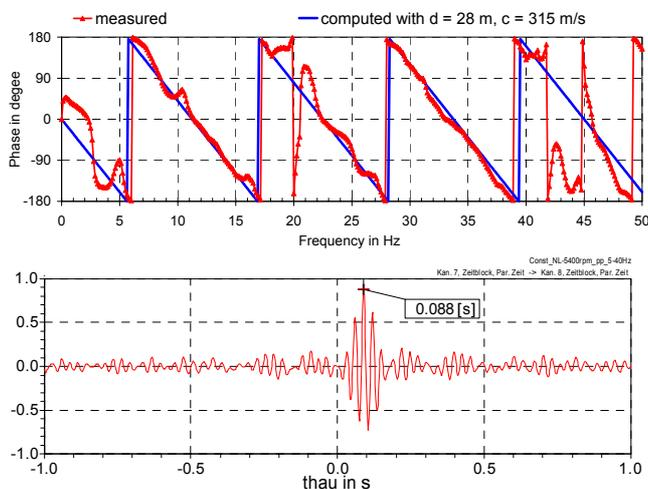
Figure 3: Measured and computed phase spectrum (top) and measured cross-correlation (bottom) from MP4 to MP3.
