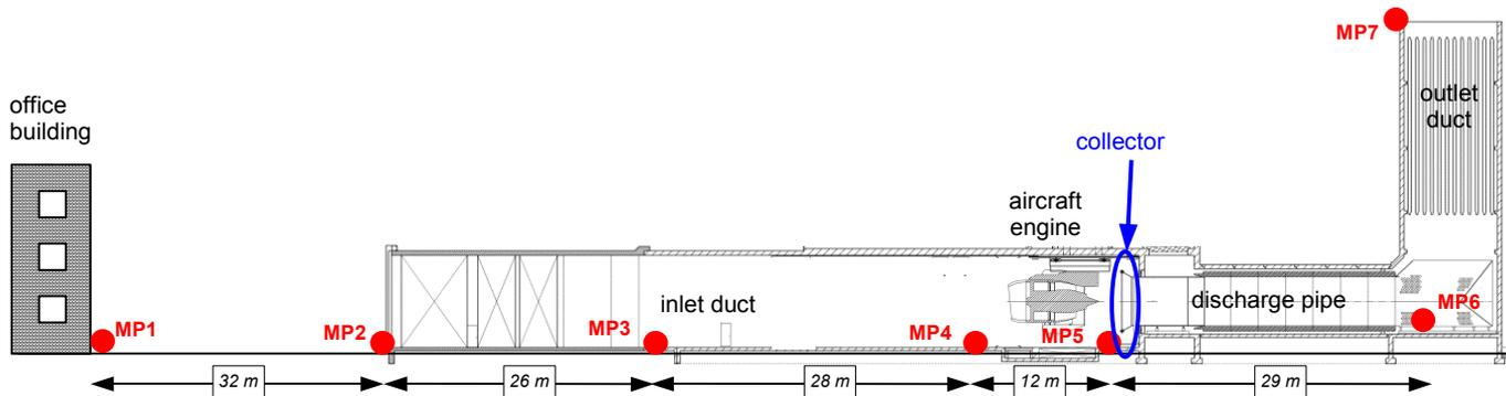
Figure 1: Test stand and microphone positions.
