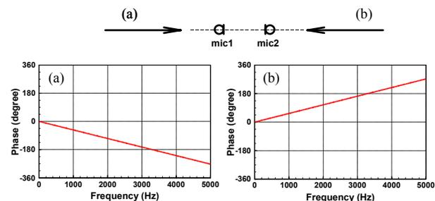
Figure 2: Detection of propagation direction using phase spectrum between two microphones.
