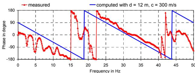
Figure 5: Measured and computed phase spectrum from MP5 to MP4.
