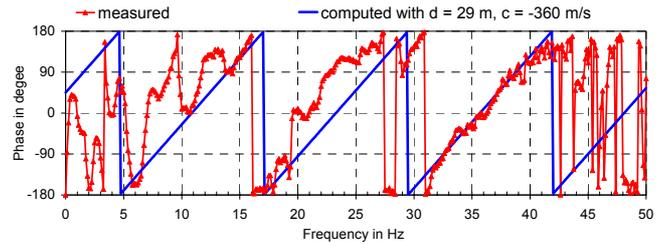
Figure 6: Measured and computed phase spectrum from MP6 to MP5.
