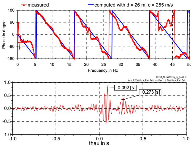
Figure 4: Measured and computed phase spectrum (top) and measured cross-correlation (bottom) from MP3 to MP2.
