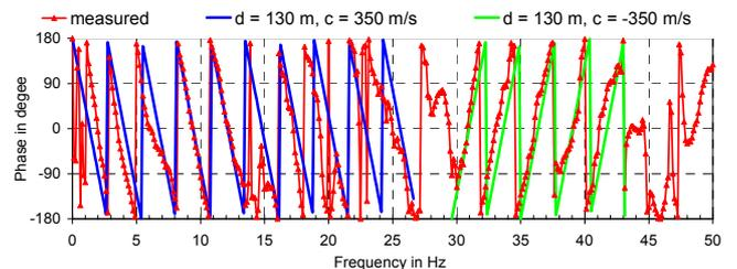
Figure 7: Measured and computed phase spectrum from MP7 to MP1.
