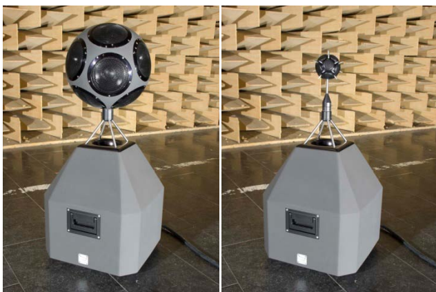
Figure 3: Measurement loudspeakers for different frequency ranges, each with 12 independently excitable membranes
