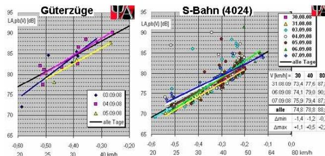
Figure 1 : daily and total average speed dependent pass-by level of freight (left) and S-Bahn trains (right)
