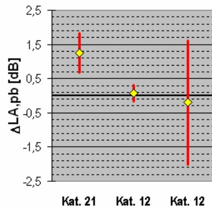
Figure 2: 95% Confidence interval of measured level difference of 3 train categories on 2 different tracks
