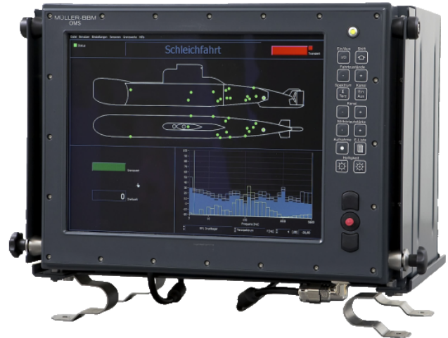
Figure 3: Operational Monitoring System
