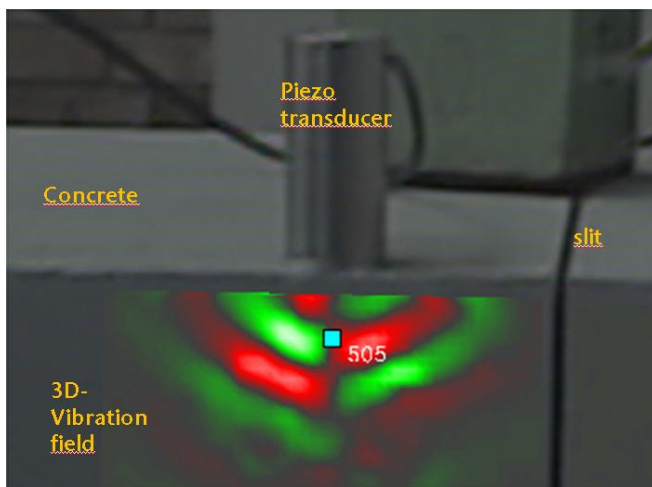
Figure 1: 3D-SLDV Visualization of sound wave propagation in concrete [1]
