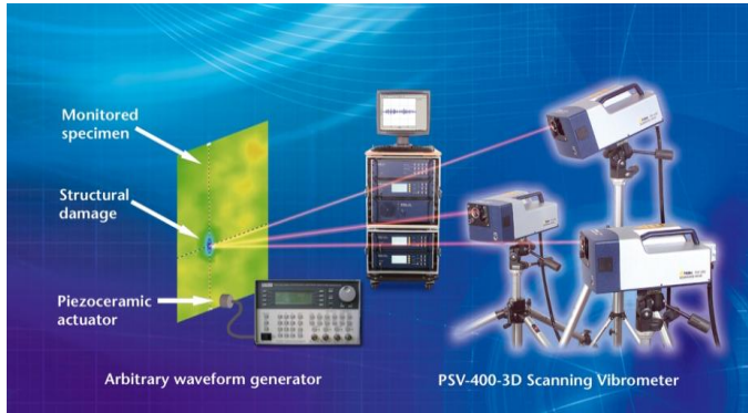
Figure 4: Experimental arrangements for Lamb-wave damage detection using 3-D laser vibrometry as a receiver.
