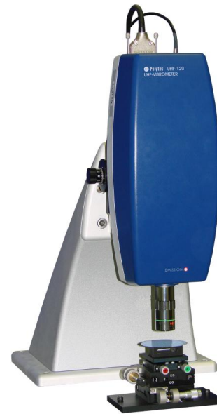
Figure 6: Ultra-High Frequency Vibrometer for measuring mechanical vibrations up to 600 MHz. [5]
