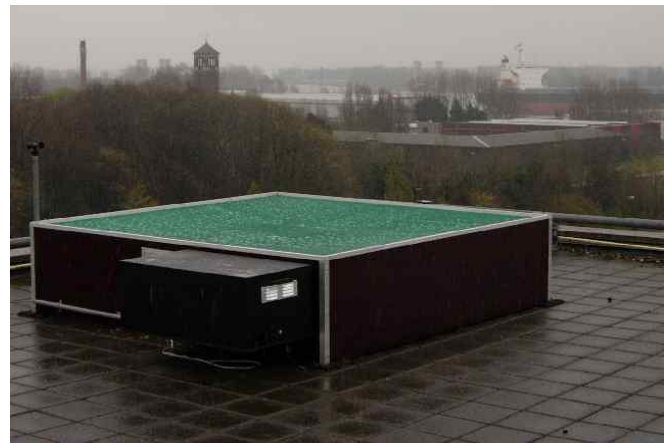
Figure 1: Aircraft noise monitoring station "Luistervink" with low microphone, sound absorbing bottom and automatic noise selection software.
