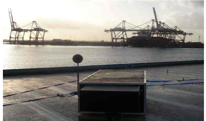
Fig 2 Industrial noise monitoring unit with auxiliary microphone inside the box.
