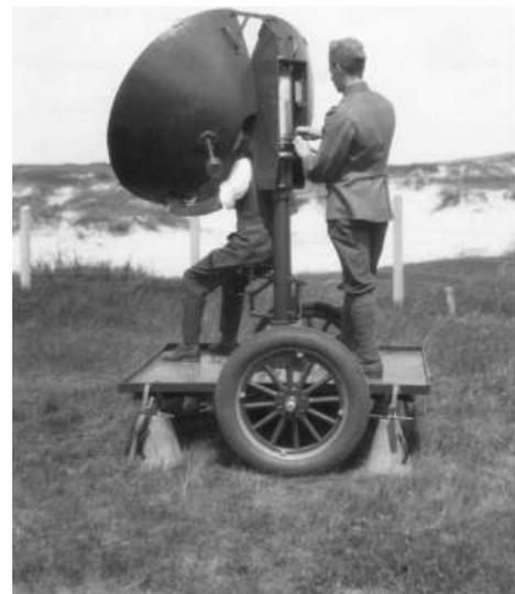
**Figure 12:** Sound locator in operation.
