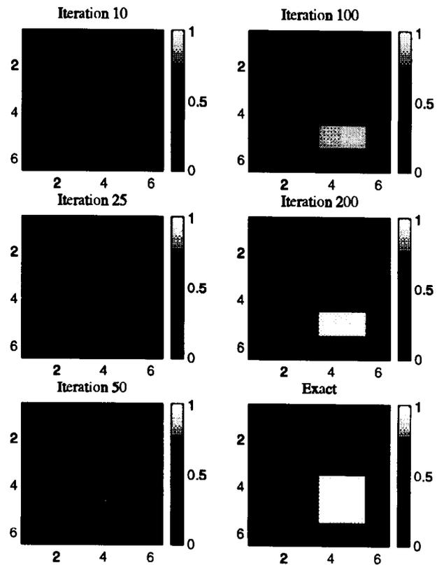
Figure 3: The gray-scale pictures of neural network reconstruction of the inhomogeneity by using the Hopfield recursive architecture.
