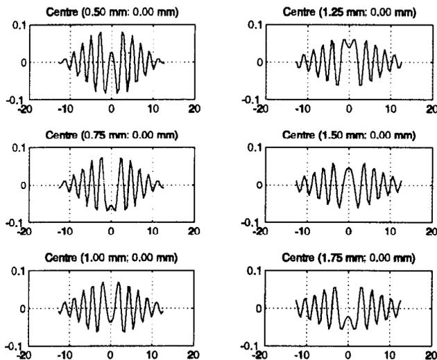
Figure 2: Real part of the scattered field in the case of plane wave irradiation of a rectangular medium-contrast object. The measuring aperture is placed at 1 mm above the interface between two fluid lossless media. The spacing between the receivers is 0.4 mm. The dimensionality of the inhomogeneity is 16 × 16 pixels. The discretisation interval is 0.1 mm.
