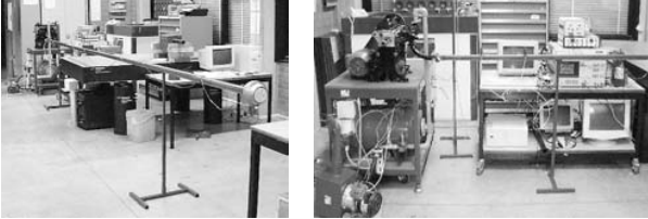
figure 4L: Measurement setup to determine the acoustical impedance of the cold engine simulator. figure 4R: The cold engine simulator connected to the measurement waveguide.
