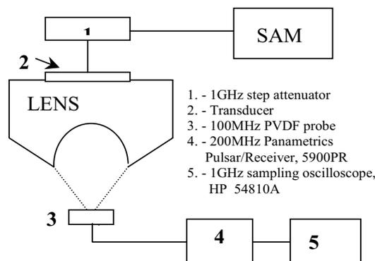
Fig. 1. The measurement system
