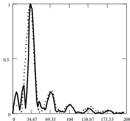
Fig.4. The experimental spectrum (dotted) and computed one (solid), averaged over the probe surface. Horizontal scale in MHz.
