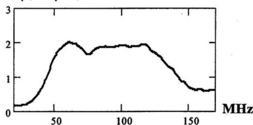
Fig.2 Frequency characteristic of the probe. Horizontal scale in MHz
