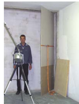
Figure 4: Gypsum board in the corner to change radiation conditions of the test wall
