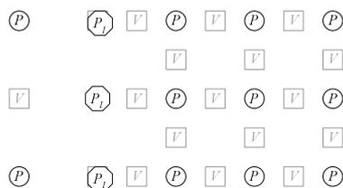
**Figure 2:** Transition from a coarse (left) to a fine segmentation (right) in an FD grid. The octagonal cells ( $P_I$ ) represent interpolators that provide pressure values to the adjacent cells of the fine grid. Two interpolators cover velocity cells of the coarse grid.
