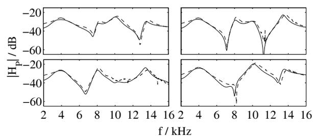
**Figure 3:** Pressure transfer functions between the artificial ear canal and four arbitrarily chosen bore holes (FD: solid line; measurement: dashed line).
