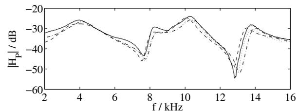
**Figure 4:** Results of the models (FD: dashed line; FE in time domain: dotted line; FE in frequency domain: dash-dotted line) and the measurement (solid line).
