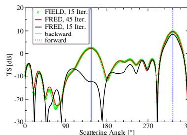
**Figure 2:** Comparison between different calculation of the target strength of a "cat's eye" with  $k\varrho = 8$ . The solid vertical line is the direction of backscattering, the dashed vertical line marks the forward scattering direction.
