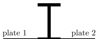
Figure 3: A line junction with I-Beam, plate: steel, 2 mm, beam flanges: steel, 4 mm, beam dimensions: 10 cm x 15 cm
