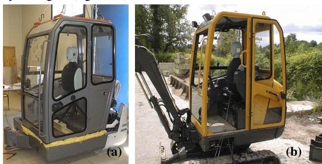
Figure 1: Studied mechanical shovel (a): studied cabin in the laboratory (b): complete machine
