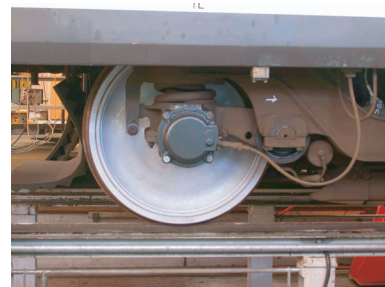
Figure 2: Measurement performed on a mounted wheel. Special painting has been applied to improve laser reflection.
