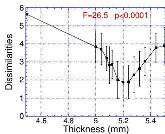
Figure 3: Dissimilarities versus constant thickness of plates
