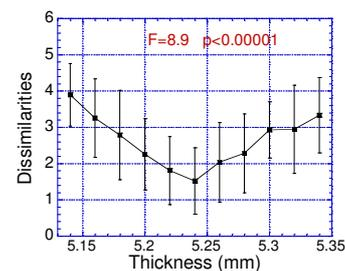
Figure 2: Dissimilarities versus constant thickness of plates
