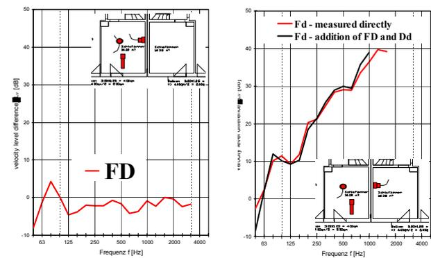
Figure 6: comparison of the addition of measured velocity level differences  $D_{v,FD} + D_{v,Dd} = D_{v,FD}$  with measured  $D_{v,FD}$  in the 1<sup>st</sup> floor. Flanking element: ceiling
