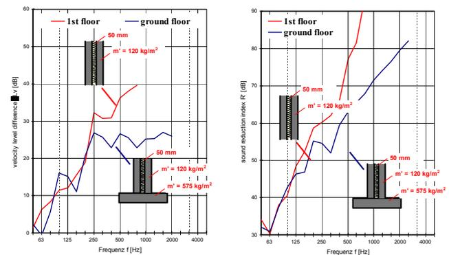
Figure 7: comparison 1<sup>st</sup> floor / ground floor left: velocity level differences for the two wall leaves right: sound reduction indices
