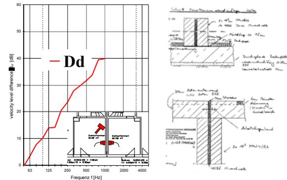
Figure 5: graph: velocity level difference  $D_{v,Dd}$  in the 1<sup>st</sup> floor draft: connection of sep. wall and ground plate / outer walls
