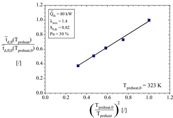
**Figure 3:** Scaling of delay times  $\bar{t}_{d,n}$  of LP flames as a function of the preheating temperature  $T_{preheat}$  of the mixture.
