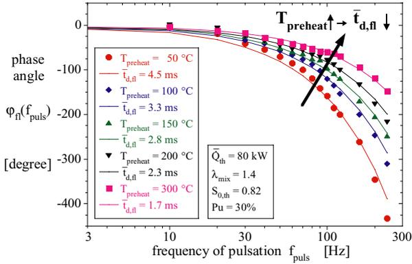
**Figure 2:** Phase angles functions  $\varphi_n(f_{puls})$  of LP swirl flames with variation of the preheating temperature  $T_{preheat}$  of the mixture.
