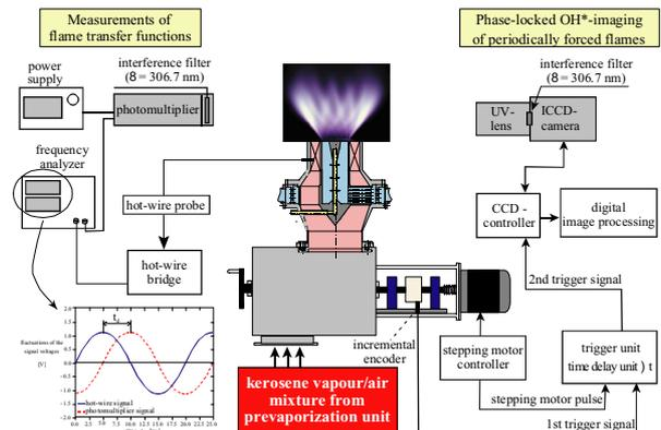
**Figure 1:** Determination of flame transfer functions and phase-correlated OH-image recording.
