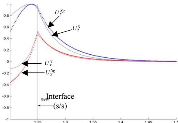
FIG 4: Generation of a Stoneley wave by a bounded beam
