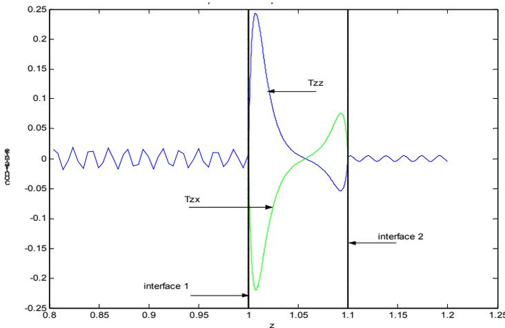
FIG 3: Real parts of stress components showing the generation of two Rayleigh waves by the bounded beam
