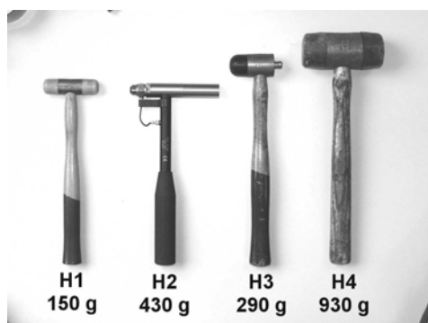
Figure 1: Hammers used for excitation of the test wall
