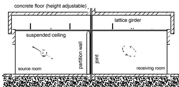
Fig. 1: test stand for suspended ceilings, height adjustable.
