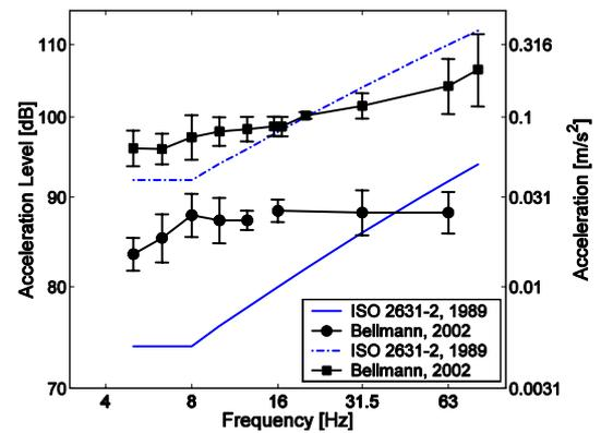
Figure 5: Measured perception threshold and equal-vibration level contours in comparison to standard data. (Adapted from [1])
