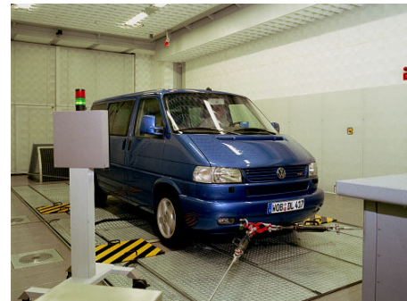
Figure 2: Four-wheel roller test bed with cooling fan.
