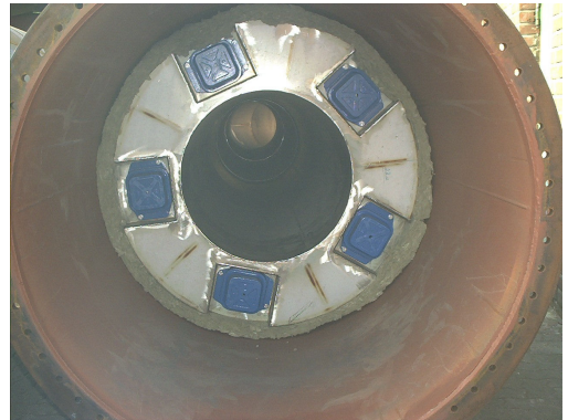
Figure 6: View to the spring elements (blue) at the CRS.
