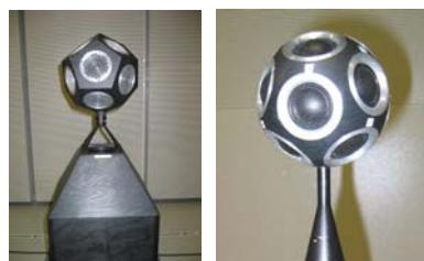
Figure 1 Monopole sound source. Mid-frequency dodecahedron ( d = 27 cm) mounted on subwoofer (left) and high-frequency dodecahedron (right, d = 16 cm)
