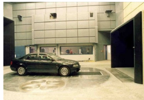
Figure 2: Plenum of the AUDI aero-acoustic wind tunnel with BCA modules as wall lining [5].
