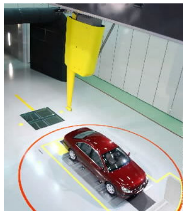
Figure 6: View to the plenum of the PSA Peugeot Citroën, Renault and CNAM aero-acoustic wind tunnel at Montigny le Bretonneux near Paris.
