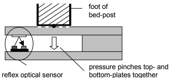
Fig 1: Schematic drawing of a sensor (side view)
