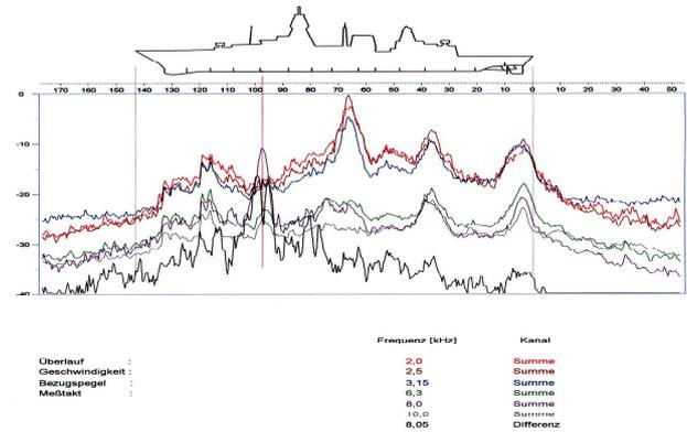
Figure 4: radiated noise sources referring to the hull measured by a linear array 30m aside the ship in 20 m depth. 1/3 octave results vers the time
