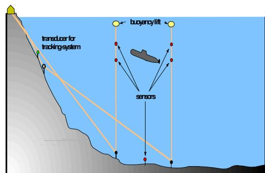
Figure 2: Sketch of the deep water range in Norway. Water depth 400m. 4 sensors are arranged in a winch system.
