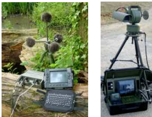
Figure 4 : PILARw system (left) composed of one (or two) tetrahedral antenna(s), a processing unit and a ruggedized display unit (laptop) and optional observation turret (PIVOT system, photo on the right).
