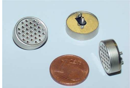
Figure 1: Miniature US transducers with 1 euro cent.
