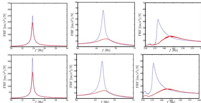
**Figure 4:** Sine-sweep FRFs (test output) with (solid line) and without (dashed line) control ( $F_{N,min} \approx 60$  N,  $1/\varepsilon = 200$ ). Top:  $F_{exc,0} = 2$  N, bottom:  $F_{exc,0} = 3$  N.
