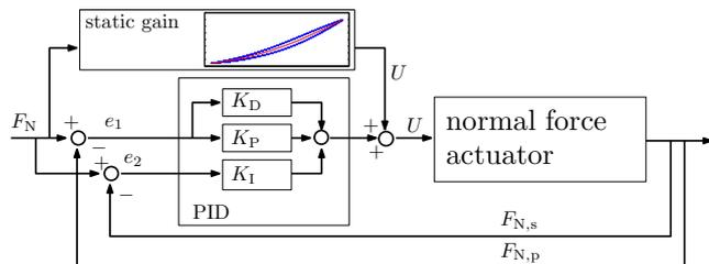
**Figure 2:** Underlying PID force control for hysteresis and drift compensation with additional static feedforward control using from measured static gain.
