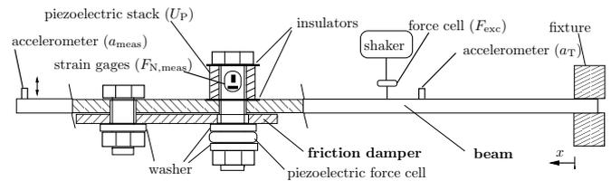
**Figure 1:** Sketch of the investigated structure with adaptive friction dampers (amplifiers not shown for sake of clarity).
