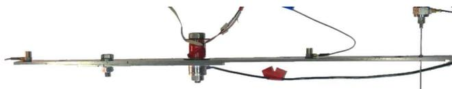
**Figure 3:** Partial view of structure with shaker stinger for excitation, friction damper with piezoelectric stack actuator for normal force adaptation, force sensor and accelerometers.
