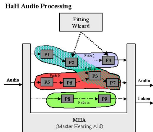
**Figure 1:** Schematic diagram of the Master Hearing Aid (MHA) framework [3]. Several signal processing blocks (P<sub>n</sub>) are combined to form processing chains.
