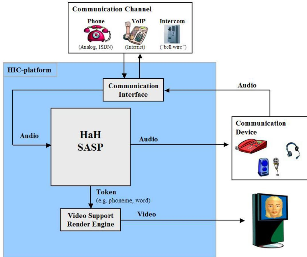
**Figure 1:** Communication scenario based on the Home Information and Communication (HIC) platform. Signals are input from different communication channels (phone, VoIP, Intercom), processed using the Supportive Audio signal Processing (SASP) and output to the communication device (e.g., headset or phone receiver). In parallel, an animated synthetic face is rendered for supporting lip-reading.
