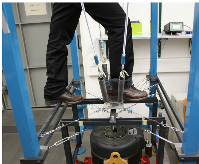
Figure 2: Mobility measurement setup to support the human body.
