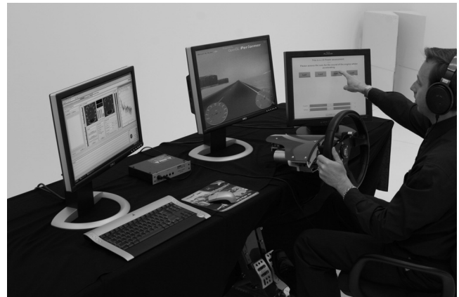
Fig.1: Desktop NVH Simulator
