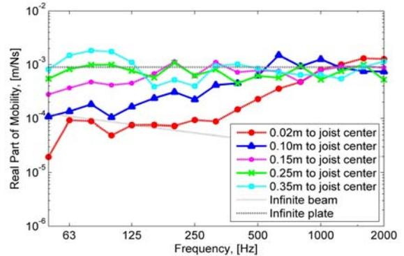
**Figure 2:** Measured real part of point mobility with parameter, distance from a joist.
