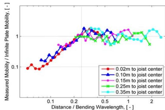
**Figure 3:** Mobilities as a function of the non-dimensional distance between drive point and nearest joist.
