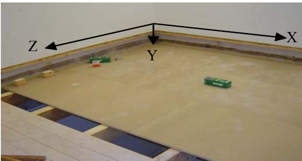
**Figure 1:** Wood joist floor, built in HfT-laboratory, used to evaluate the spatial dependence of drive point mobility
