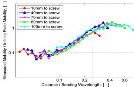
**Figure 4:** Point mobility as a function of the non-dimensional distance between the drive point and adjacent fixing point.
