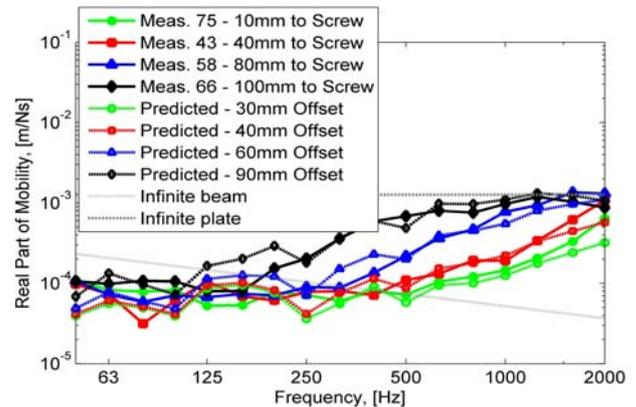
**Figure 5:** Measured and predicted real part of the drive point mobility for points located above a joist as a function of distance from a screw.
