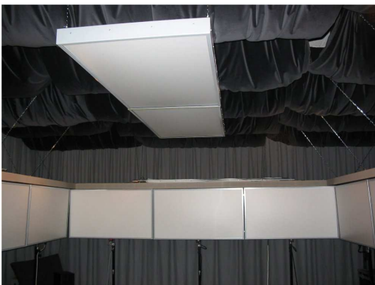
Figure 1: The Wave Field Synthesis test setup at the TU Delft, including the ceiling array.
