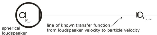
**Fig. 2:** Measurement set up for the small sphere low frequency calibration ( $f < 500 \sim 1\text{kHz}$ ).
