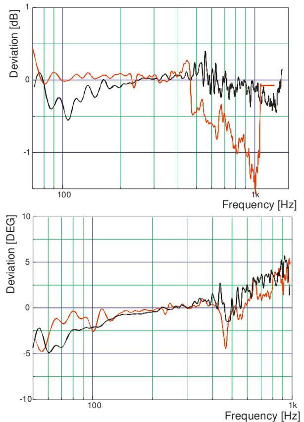
**Fig. 3:** Deviation between short standing wave tube and LF sphere calibration. Pressure probe is put so that the membrane is close to the internal surface of the sphere. Red: large sphere, black: small sphere. Upper: difference is dB, lower: difference in degrees.
