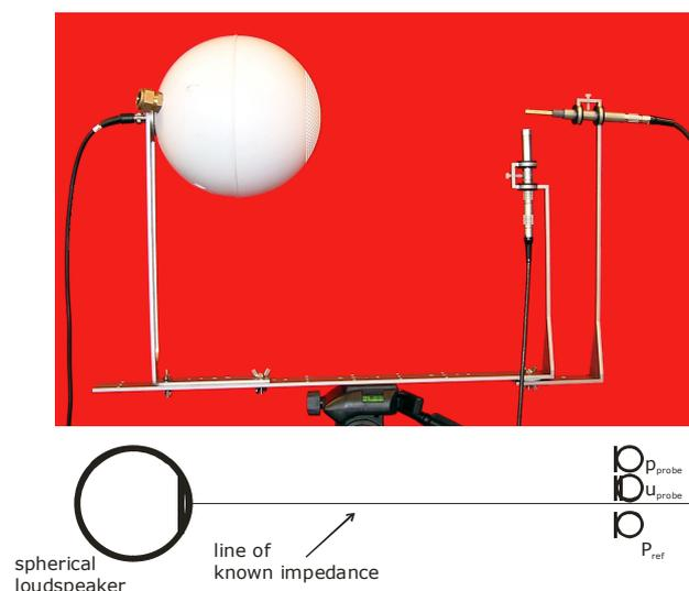
**Fig. 1:** Measurement set up for the 'piston in a sphere' high frequency calibration ( $f > 50-100\text{Hz}$ ).
